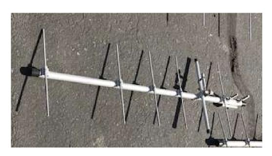
Cushcraft A449-11S 11 Element Yagi 440 - 450 (used. I have 2...one is complete and one has a broken reflector element which can easily be repaired)
